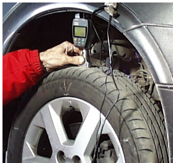
Tyre edge wear measurement
